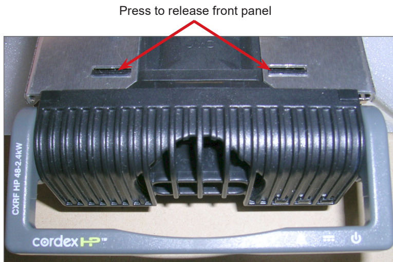
Figure 17 — Removing Front Panel from Rectifier
