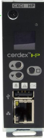
2. Pull here to remove the controller from the shelf.
